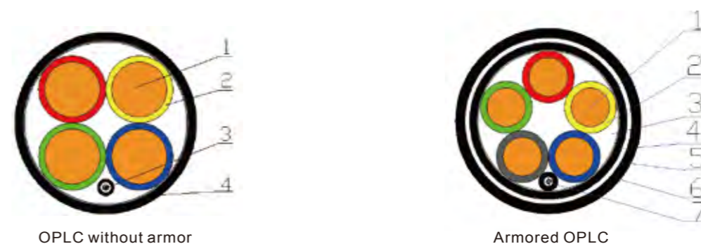
Figure 1 1 – conductor 2 – insulation 3 – optical unit 4 – sheath
